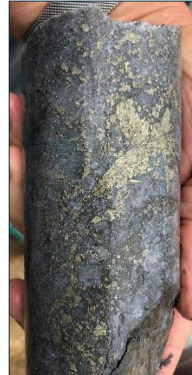
B veins, LMDD002, 723.2m LMDD002, 890.5m, coarse grained chalcopyrite + pyrite
