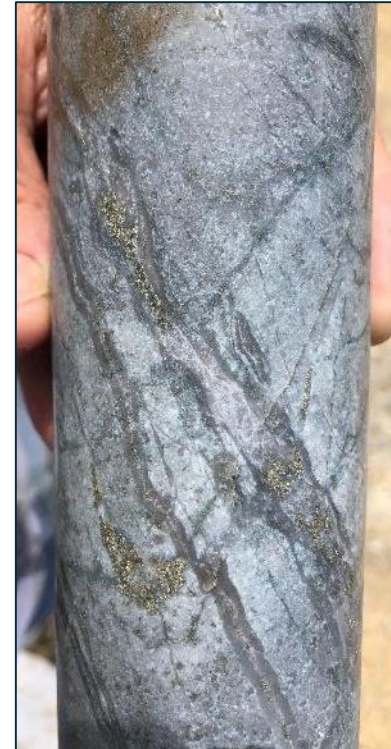
B veins, LMDD002, 723.2m LMDD002, 890.5m, coarse grained chalcopyrite + pyrite
