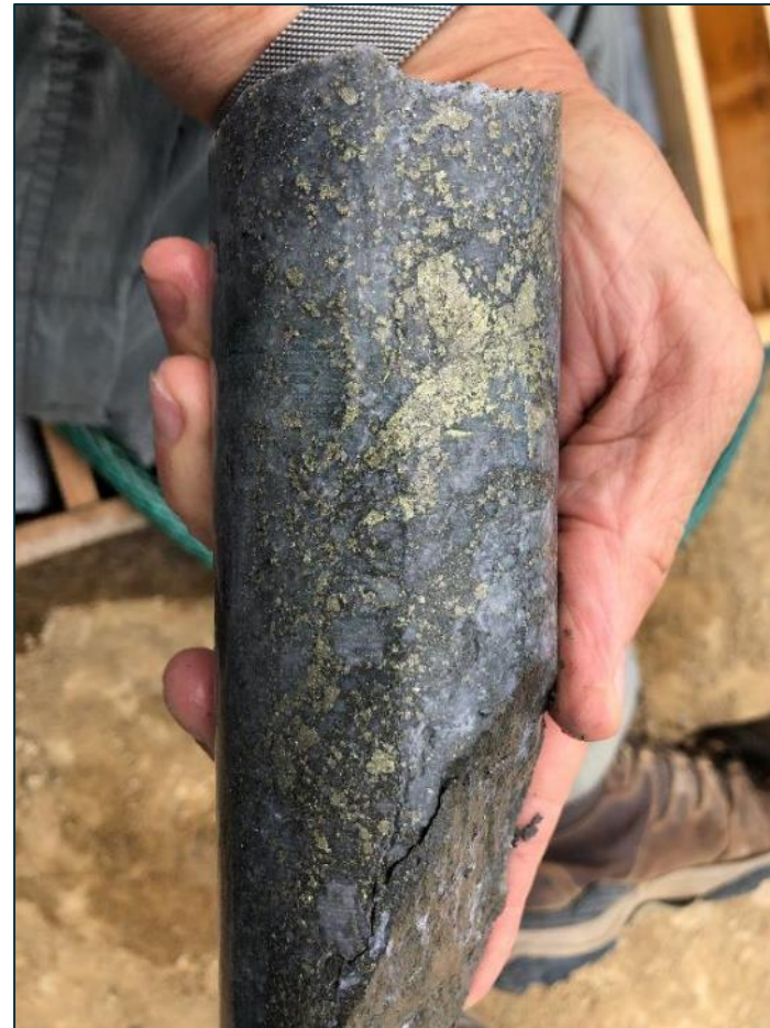
LMDD002, 890.5m, coarse grained chalcopyrite + pyrite
