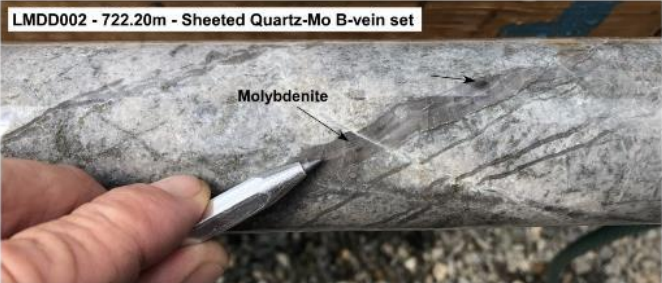
Variety of porphyry B-vein textures seen in LMDD002 (Cpy = chalcopyrite).
