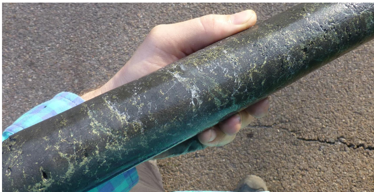
Figure 3: Drill core from hole VDD 193 at approximately 576.7m to 577m down hole, showing stringer and blebby chalcopyrite in magnetite.
