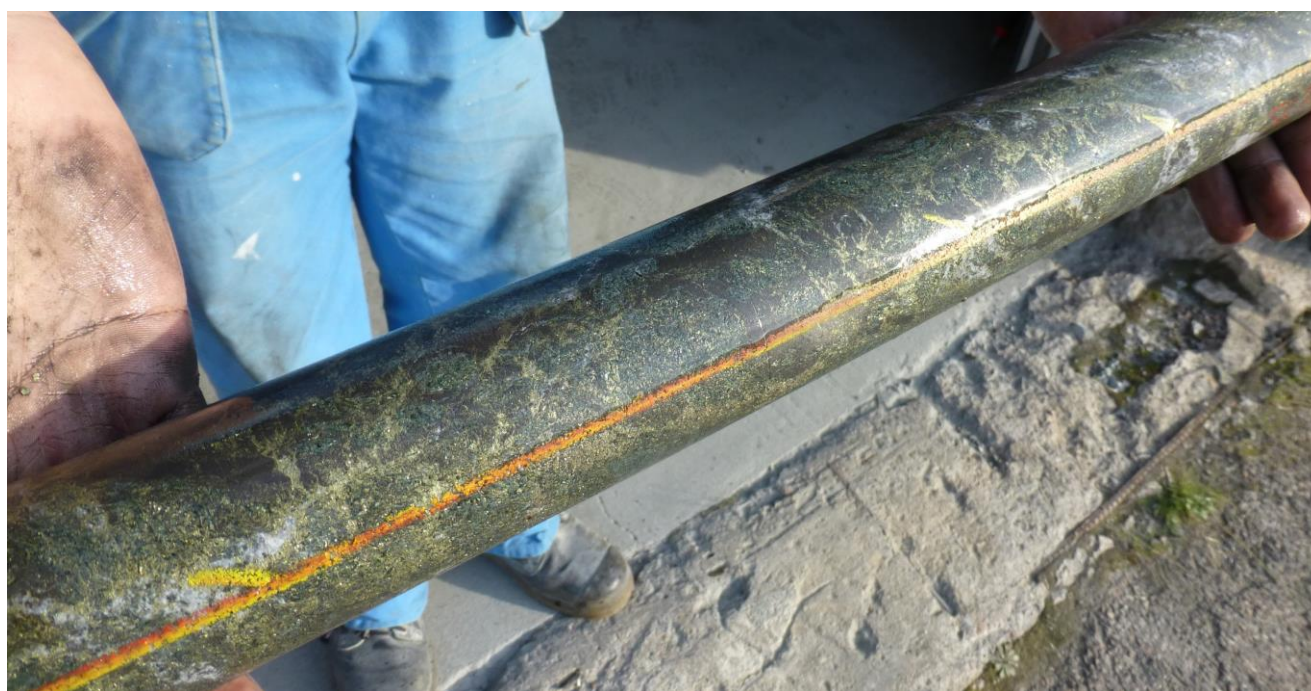
Figure 2: Drill core from hole VDD 193 at approximately 567.45m to 567.9m down hole, showing stringer and semi-massive chalcopyrite in magnetite.
