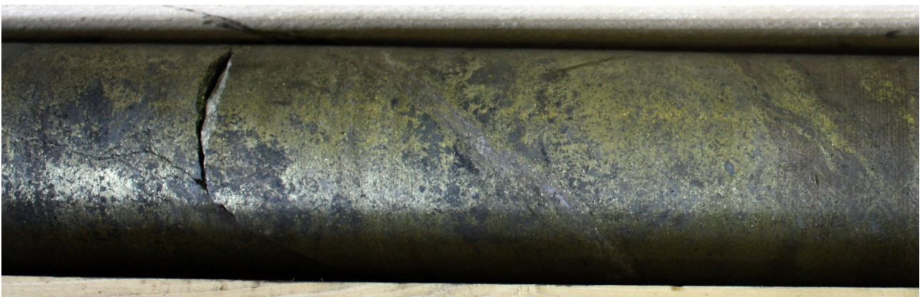
Figure Three - Massive Sulphide Mineralisation Intersected in Drill Hole VDD0127 (yellow sulphide = chalcopyrite; brown sulphide = pyrrhotite)
